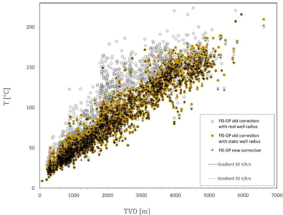
**Figure 3:** The formation temperatures determined from the corrected BHT values are plotted against the depth. Crosses refer to the new correction. Grey circles refer to the old correction if a fixed radius would have been used. Brown discs show corrected BHTs before the new correction method was introduced.
