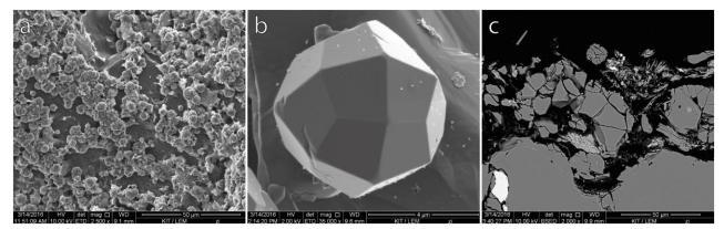
Figure 2: SEM images (SE and BSE) of analcime precipitation on sandstone sample after 260 °C experiments: (a) sample surface is covered by euhedral analcime (TenSst), (b) spherical analcime on PfSst, (c) BSE thin section image (PfSst) with partly dissolved sandstone matrix, quartz grains and secondary analcime.
