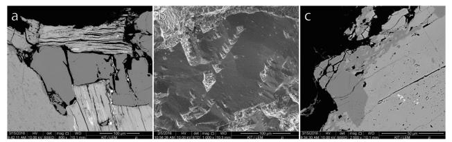
Figure 1: SEM images (SE and BSE) of the granite sample after 260 °C experiment: (a) disintegrated rock fabric due to chloritization of biotite and quartz dissolution (dark grey); (b) triangular etch pits on the quartz surface; (c) albitization of K-feldspar at the mineral-fluid interface.
