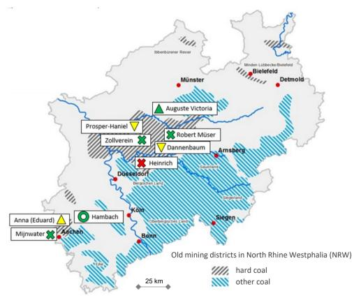
Figure 9: Project locations for mine water use in NRW and Heerlen (modified from district government of Arnsberg, 2016). Legend: O- sump pit drainage, in service; ▲ - borehole heat exchanger, in planning stage; ▲ - borehole heat exchanger, in service; ▼ - heat storage, in planning stage; × - mine water drainage, inoperative; × - mine water drainage, in service
