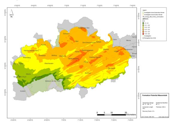
Figure 8: Geothermal potential of Devonian limestone referred as *Massenkalk* with more than 300 m thickness, in 3,000 to 7,000 m depth, in temperature range of 80°-180°C (after Bracke et al., 2016)
