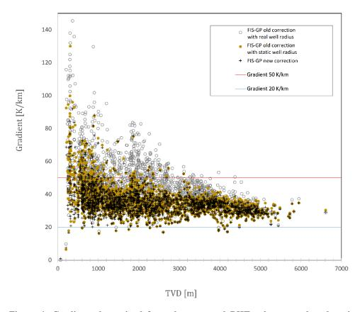
Figure 4: Gradients determined from the corrected BHT values are plotted against the depth. The strong scattering for depths less than 500 m is partly due to the fact that small changes in temperature cause large changes in the gradient.
