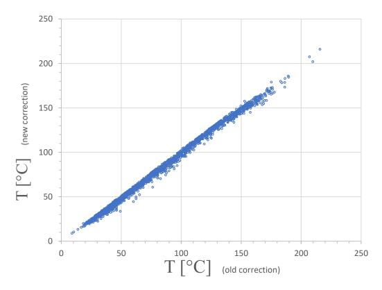
Figure 2: Comparison of the old and new correction procedure for BHT values with only one shut-in time at one depth.
