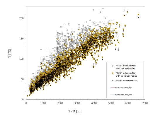
Figure 3: The formation temperatures determined from the corrected BHT values are plotted against the depth. Crosses refer to the new correction. Grey circles refer to the old correction if a fixed radius would have been used. Brown discs show corrected BHTs before the new correction method was introduced.
