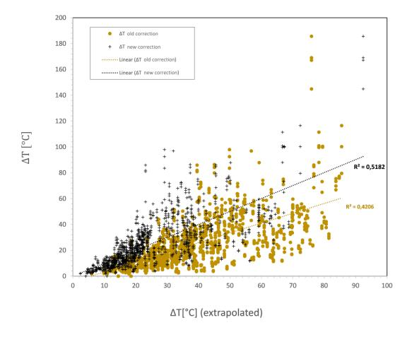
Fig. 1:  $\Delta T$  values calculated according to formula 4 (crosses) and formula 2 (circles) plotted against extrapolated  $\Delta T$  values from a sequence of 3 or more BHT measured values (cylinder source model approach).
