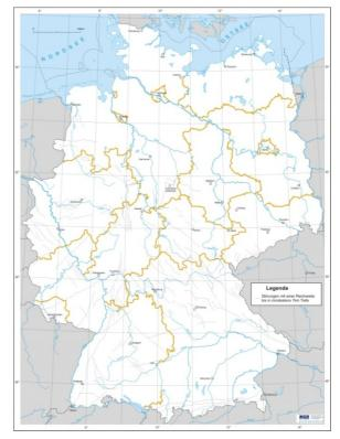
Figure 2: Deep-seated fault systems with a possible extension up to 7 km depth.
