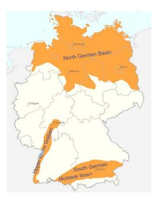
Figure 1: Areas with potential for hydrogeothermal exploitation in Germany (Pester et al. 2010). From North to South: Upper Rotliegend (Upper Permian) sandstone aquifer in the North German Basin; Upper Muschelkalk and Buntsandstein (Middle and Early Triassic) aquifers of the Upper Rhine Graben; Malmkarst (Upper Jurassic) aquifer in the South German Molasse Basin.
